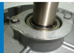
Internally locked drive-end bearing construction
