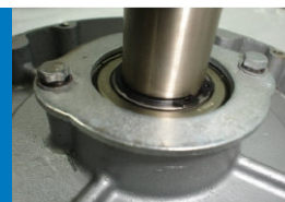
Internally locked drive-end bearing construction
